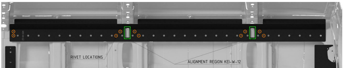
Figure 5. Fit above KEI-W-9; use every highlighted rivet hole.
