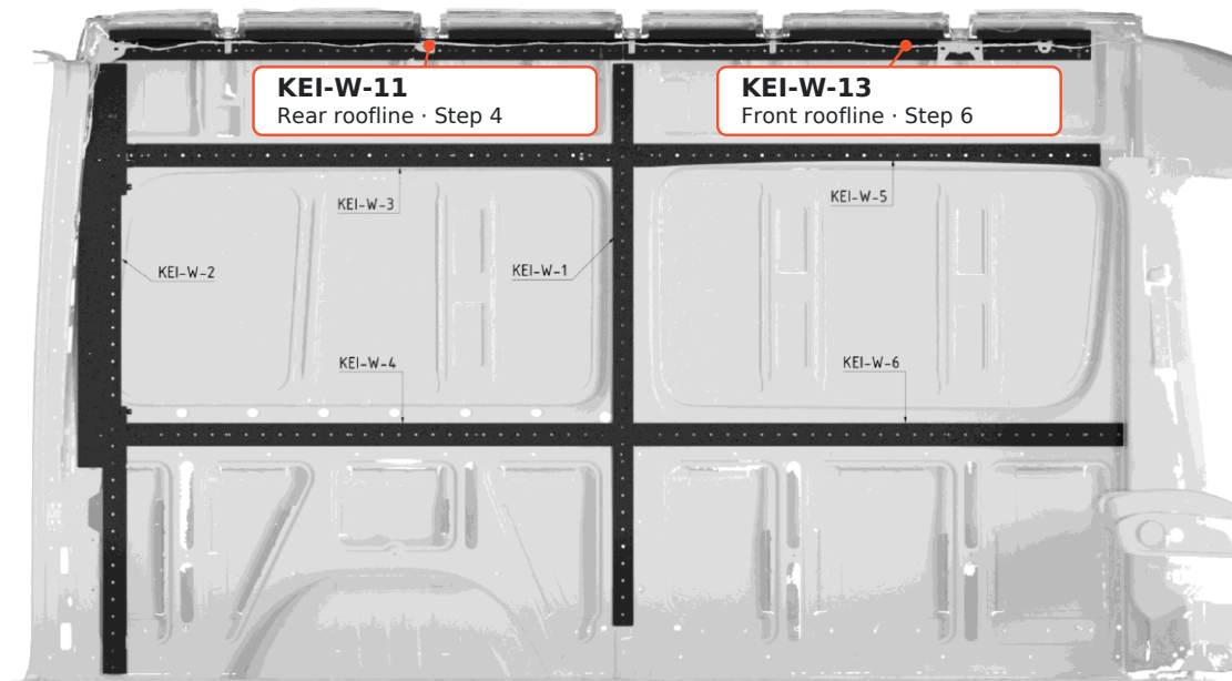
Figure 1 — Driver side. Front of van: right. KEI-W-11 and KEI-W-13 are fitted in Steps 4 and 6.
