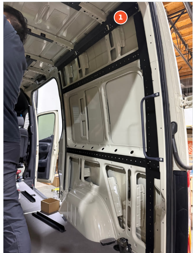
1 — Roofline anchor rail
