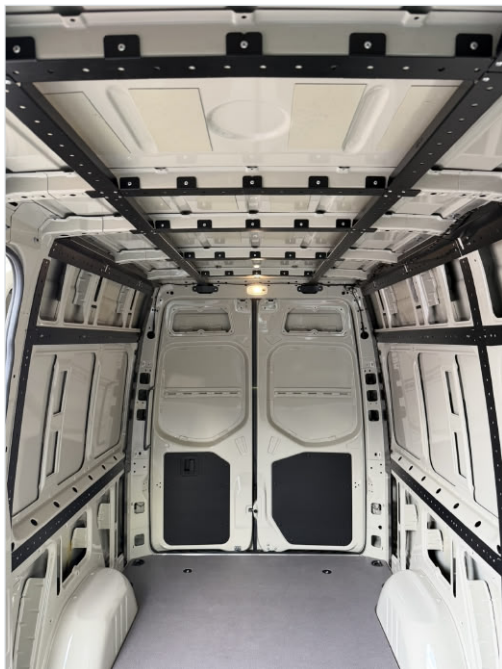
Figure 10 — 680 mm spacing and ceiling rivet holes. Use the diagram's measuring points; the photos are fit references.
